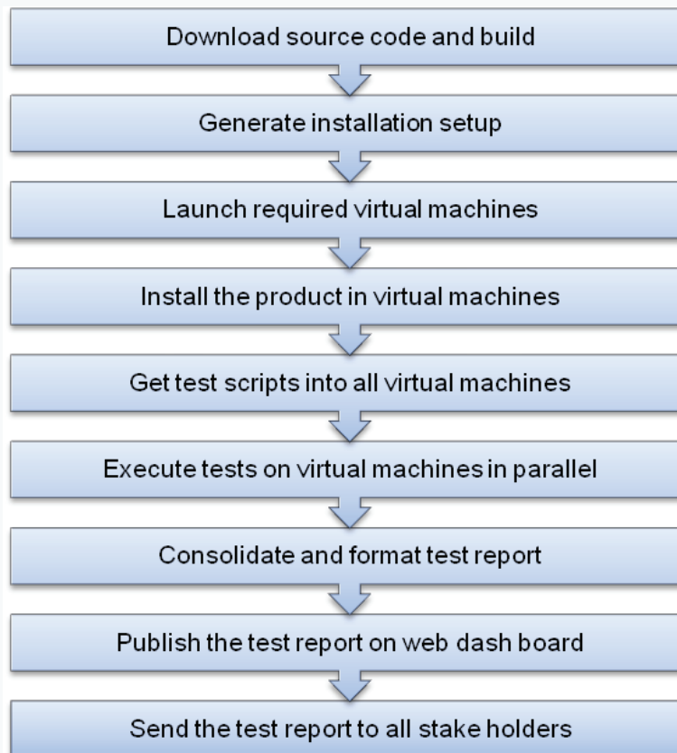
Figure 3: CIVIM work flow
